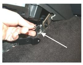
Attach frame support bracket (#4) to vehicle using 10/32 x ½" phillips machine screws, washers, and keps nuts
